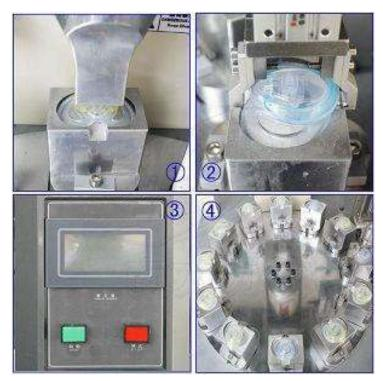
Touch screen, parameter set intuitional and exact; Computer control system of dual language, high anti-interference ability, time accuracy is up to 0.01 seconds and easy to adjust;
